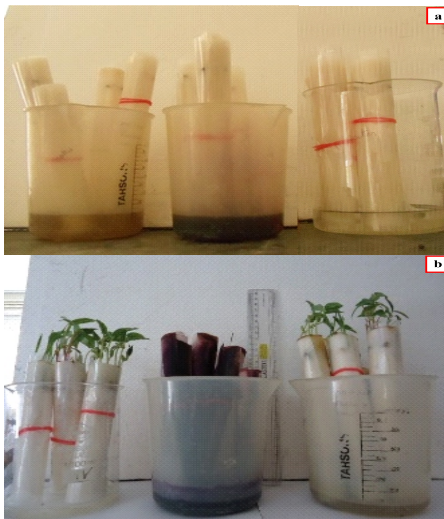
Plate 1: Effect of textile dyeing effluent on germination and growth of selected cereals ( Triticum vulgare and Oryza sativa ) and pulses ( Vigna radiata and Vigna mungo ) by roll towel method (a1) treated effluent (a2) raw textile dyeing effluent and (a3) control- water on day 1 and (b) set ups on day 5
